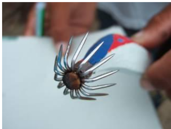
Figure 13 Turlutte - The pronged head of the lure designed for catching squid. These lures were introduced by AO/MAG/97/008 project.
