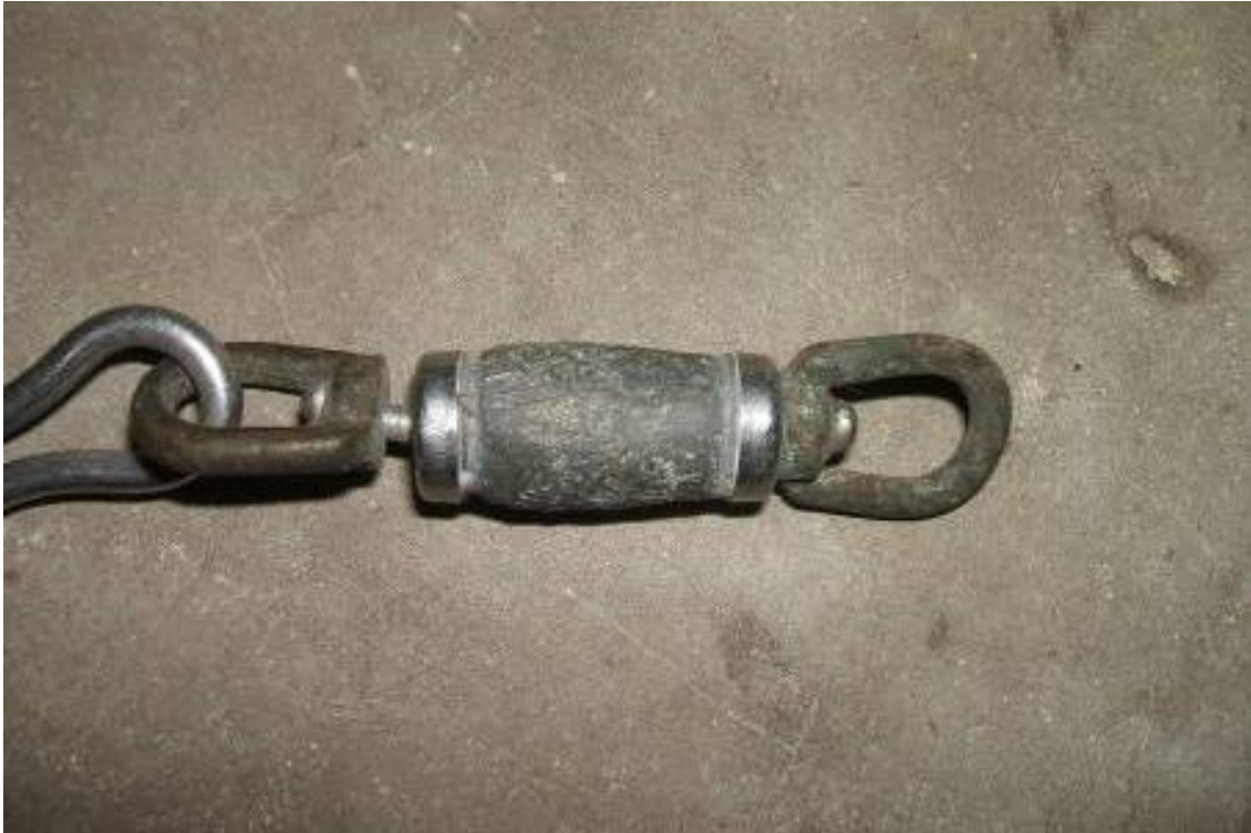
Figure 10 Koro - A barrel swivel link to prevent the line from twisting
